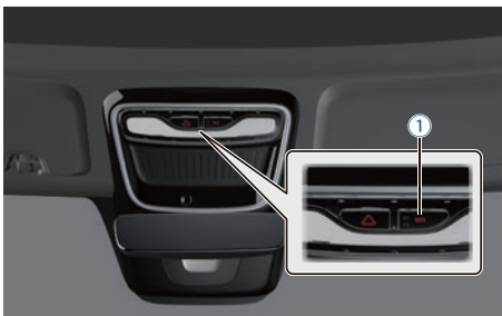
1. Emergency call switch
