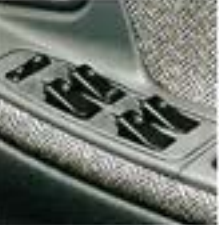
The pull-up design of the power window switches reflects Mazda's commitment to safety. A window closes only when the button is pulled up, thus eliminating the danger of a child being trapped by the neck should the button be pressed unintentionally.
